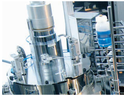
Bond module with automatic, low-force wedge error compensation, optional with alignment within bond chamber
