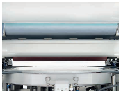
Detape module for removing temporary bonding adhesives by peeling it off with an adhesive tape
