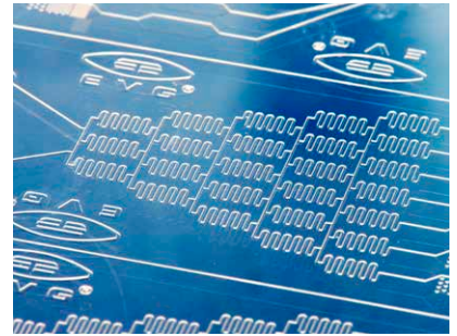
Microfluidic chips replicated in PMMA by hot embossing Source: EVG
